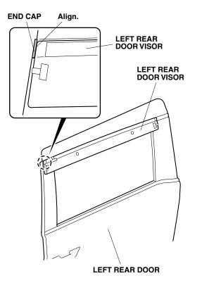
While applying light pressure against the left rear door visor, carefully remove the adhesive backings. Push up on the rear brackets while removing the adhesive backings.
