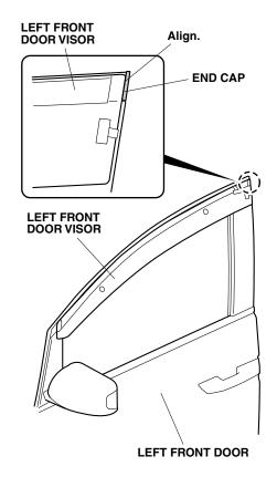
While applying light pressure against the left front door visor, carefully remove the adhesive backings. Push up on the front brackets while removing the adhesive backings.
