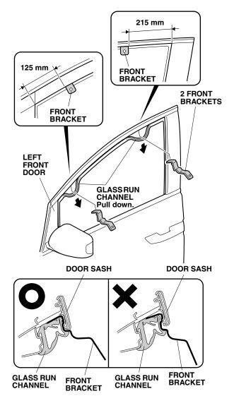
3. Reinstall the glass run channel to secure the two front brackets. Be sure the brackets are installed tightly to the door sash, and that the glass run channel is properly seated.
