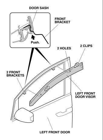
7. Secure the left front door visor to the front brackets with two clips. Push up on the front brackets while installing the two clips. Install the clips correctly, they cannot be removed.
