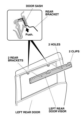
17. Secure the left rear door visor to the front brackets with two clips. Push up on the rear brackets while installing the two clips. Install the clips correctly, they cannot be removed.
